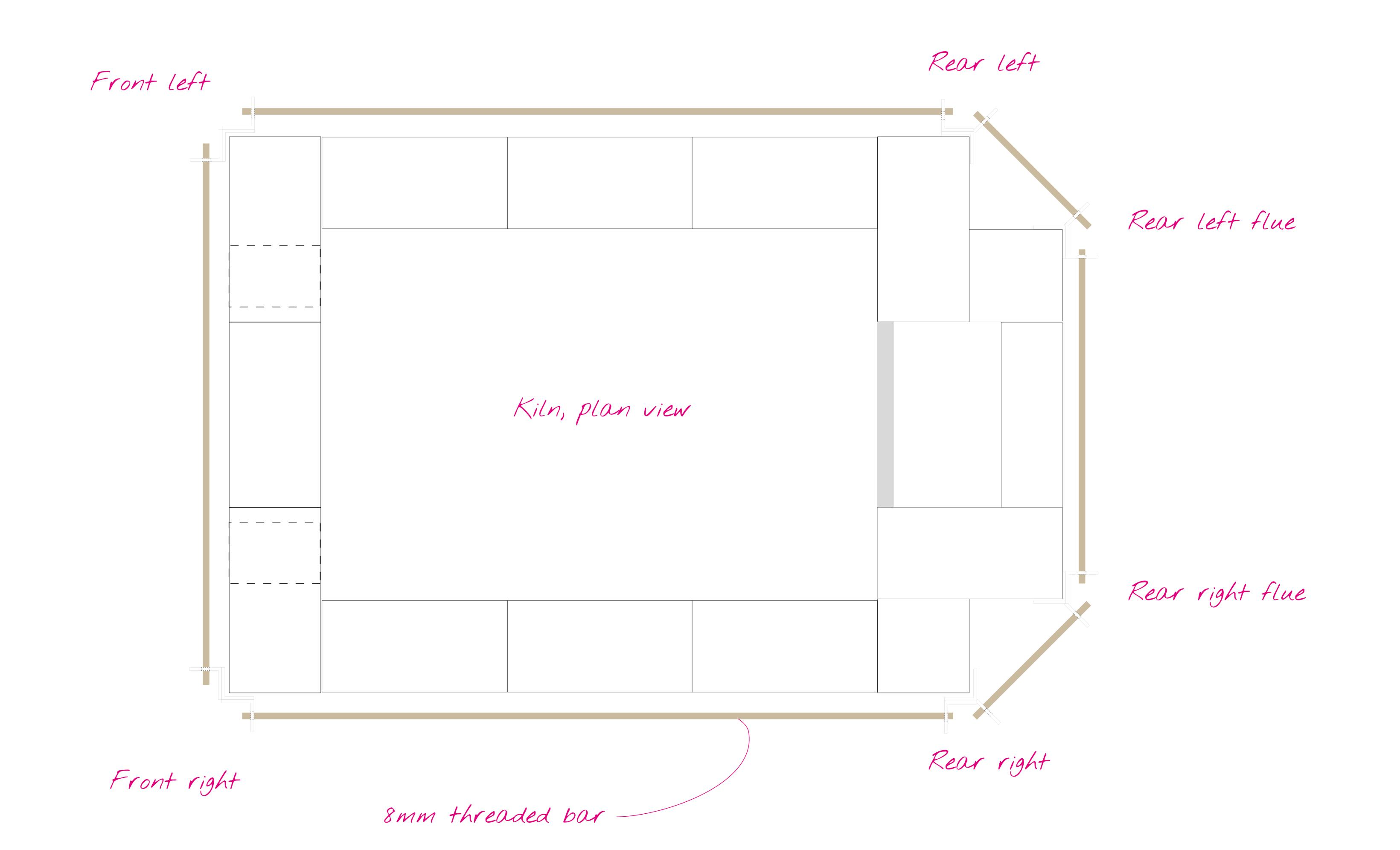
Kiln above is loose lined bricks so they can move about a little with expansion and contraction under extreme heat. The walls have tiny gaps between the bricks and whilst reasonably stable as-is securing with steels and threaded be will make it more stable and enable the structure to be compressed, removing the gaps and enabling ongoing adjustments
